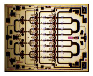
The TriQuint TGA1082B-EPU is a three stage HPA MMIC design using TriQuint's proven 0.25 um Power pHEMT process. The TGA1082B is designed to support a variety of millimeter wave applications including point-to-point digital radio and LMDS/LMCS and Ka band satellite ground terminals.
