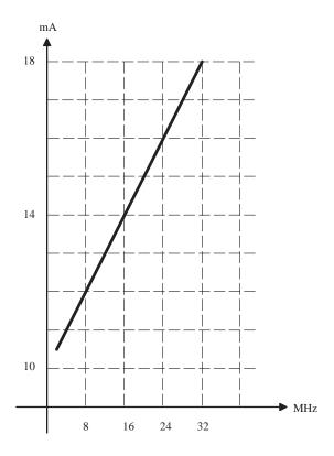
$\label{eq:control} \mbox{Figure 33. I}_{CC} \mbox{ Versus Clock Frequency} \\ \mbox{ at 250 KTimeslot/s}$
