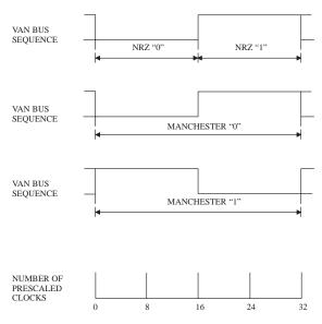
Figure 11. Data Encoding.
