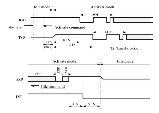
Figure 30. Idle and activate timings
