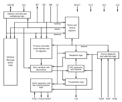
Figure 1. Block Diagram
