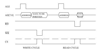
Figure 4. INTEL Read and Write Cycles.
