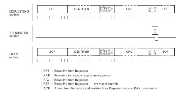
Figure 15. Reply Request Frame with Deffered Reply
