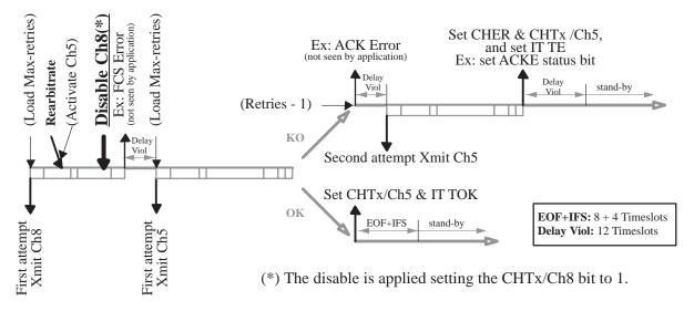
Figure 28. Disable channel after rearbitrate example
