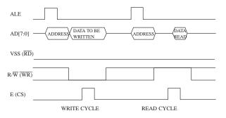
Figure 5. MOTOROLA Read and Write Cycles.
