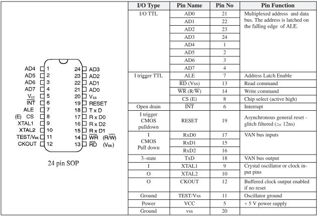
Figure 2. Pinout
