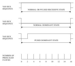
Figure 7. State Encoding.
