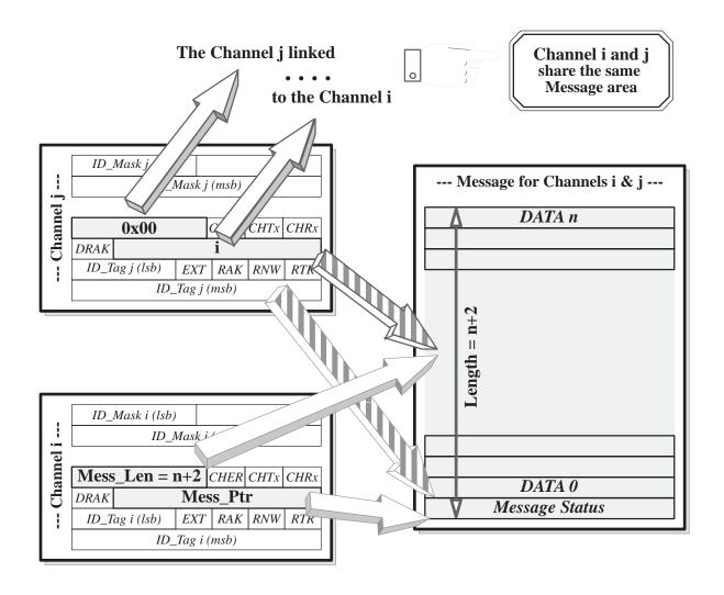
Figure 31. Linkage mechanism
