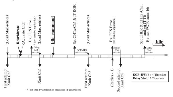
Figure 27. Idle and rearbitrate example
