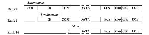
Figure 9. Hierarchical Access Methods
