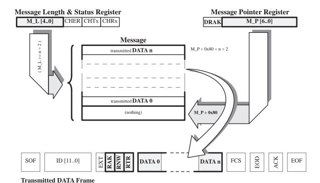
Figure 23. Message buffer structure for transmission
