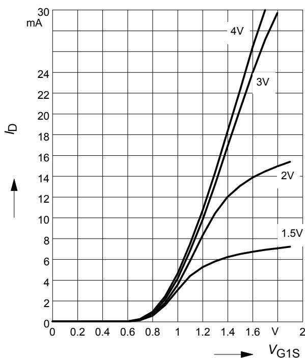
**Drain current  $I_D = f(V_{GG})$**
