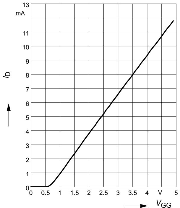
**Drain current  $I_D = f(V_{GG})$**
