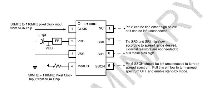
Note: To set the P1708C to standby mode, disable the input clock (pin 1 CLKIN) and pull SSON (pin 5) low. *Refer Standby Mode Selection Table.*
