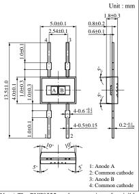
Note) The PNZ0322 package consists of a visible light cutoff resin. Therefore the chips (A and B) shown in the drawing cannot actually be seen.
