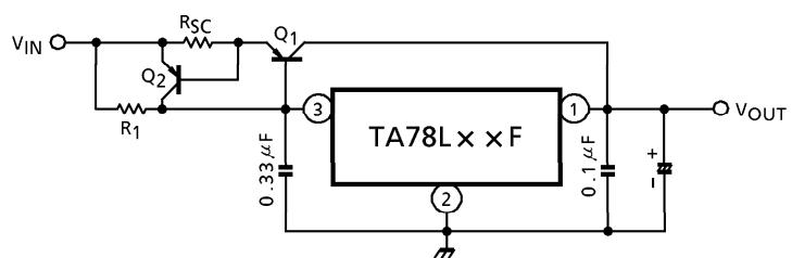
$$R_{SC} = \frac{V_{BE2}}{I_{SC}}$$
