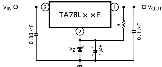
$V_{OUT} = V_Z + V_{OUT}$  (of IC)
