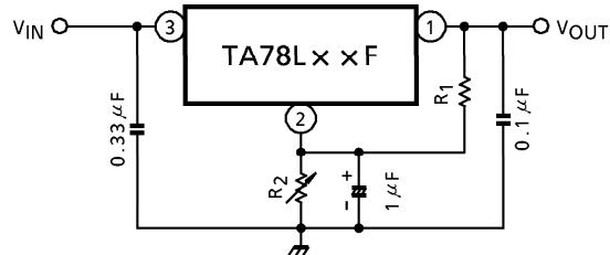
$$V_{OUT} = R_2(I_B + \frac{V_{OUT}(\text{of IC})}{R_1}) + V_{OUT}(\text{of IC})$$
