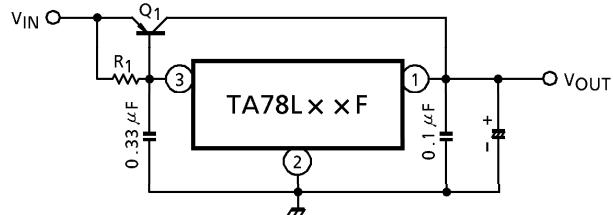
Use a required radiation plate for Q<sub>1</sub>.
