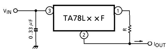
$$I_{OUT} = \frac{V_{OUT}}{R} + I_B$$
