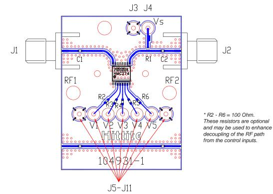
The circuit board used in the final application should use RF circuit design techniques. Signal lines should have 50 ohm impedance while the package ground leads should be connected directly to the ground plane similar to that shown below. A sufficient number of VIA holes should be used to connect the top and bottom ground planes. The evaluation circuit board as shown is available from Hittite Microwave Corporation upon request.
