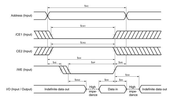
Cautions 1. During address transition, at least one of pins /CE1, CE2, /WE should be inactivated.
