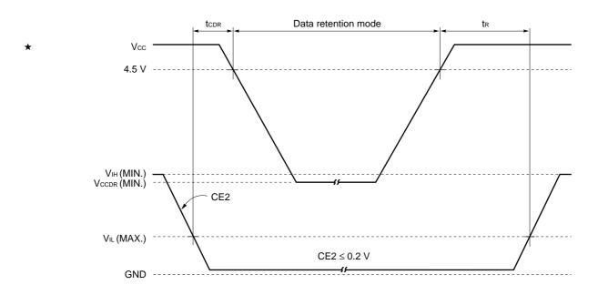
**Remark** On the data retention mode by controlling CE2, the other pins (/CE1, Address, I/O, /WE) can be in high impedance state.
