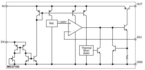
MIC37102 Adjustable Regulator Block Diagram
