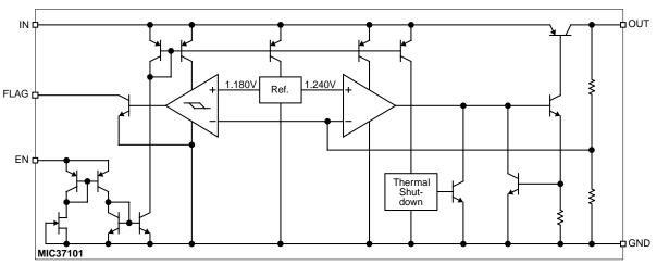
MIC37101 Fixed Regulator with Flag and Enable Block Diagram
