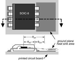
Figure 3. Thermal Resistance
