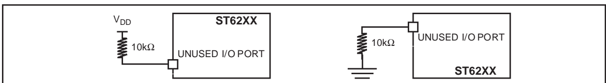
Figure 62. Two typical Applications with unused I/O Pin
