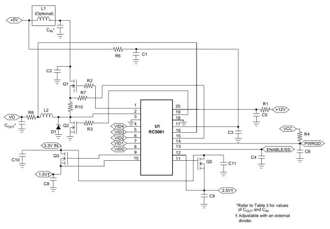
Figure 2. Application Circuit for Coppermine/Camino Motherboards (Typical Design)
