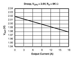
CPU Output Voltage vs. Output Current
