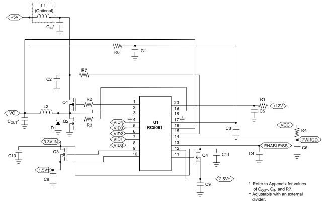
Figure 1. Typical Application Circuit (Worst Case Analyzed! See Appendix for Details) (Components based on Worst Case Analysis—See Appendix for Details)
