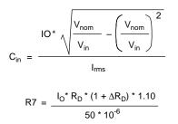
The value of R7 must be  $\leq 8.3$ K $\Omega$ . If a greater value is calculated, R<sub>D</sub> must be reduced.
