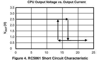
The converter exhibits a normal load regulation characteristic until the voltage across the MOSFET exceeds the internal short circuit threshold of  $50\mu A * 8.2K\Omega = 410mV$ , which occurs at  $410mV/25m\Omega = 16.4A$ . (Note that this current limit level can be as high as  $410mV/15m\Omega = 27A$ , if the MOSFET has typical R<sub>DS,on</sub> rather than maximum, and is at  $25^{\circ}C$ ).
