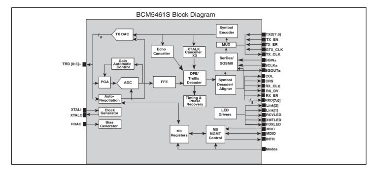
The BCM5461S is a fully integrated 10/100/1000BASE-T Gigabit Ethernet transceiver optimized for low power and small footprint size to enable backplane and uplink applications. By lowering system cost and reducing power dissipation by nearly 30%, the BCM5461S enables a new class of cost-effective Gigabit Ethernet equipment, driving the delivery of Gigabit bandwidth to the desktop.
