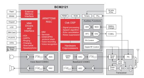
The **BCM2121** GPRS/GSM baseband processor offers a high level of system integration, performance, and features for next-generation handsets and radio cards. The **BCM2121** is a single-chip baseband device that is applicable for wireless handsets and speakerphones.
